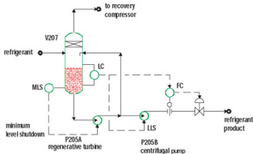
**Figure 1:** The control scheme uses low-liquid-level shutdown (LLS) to turn the centrifugal pump off when it is not needed, and minimum-liquid-level shutdown (MLS) to protect the turbine.
