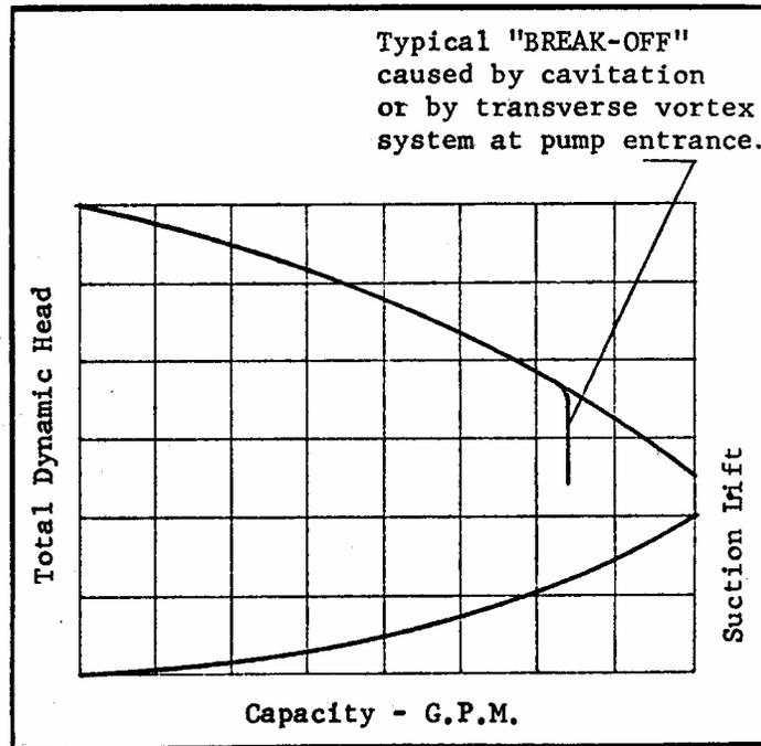
Figure 1. Normal axial flow was momentarily disrupted with each occurrence of a vortex. The performance graph shows this as a "break-off" similar to that caused by cavitation.
