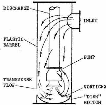
Figure 3. Flow pattern for a barrel with a dish bottom.
