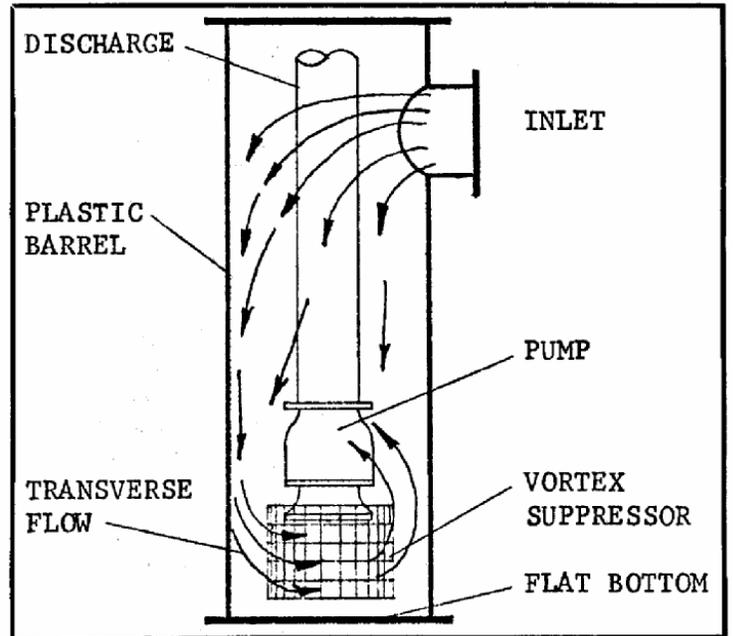
Figure 7. Use of grid system prevents the occurrence of vortices in barrel flow pattern.
