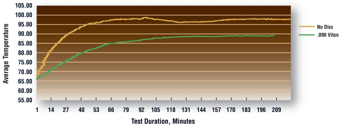
Fig. 3. Flinger disc tests, ISO Grade 68, 3,600 rpm, Average Temp. vs. Time (Source [www.tricomfg.com](http://www.tricomfg.com))
