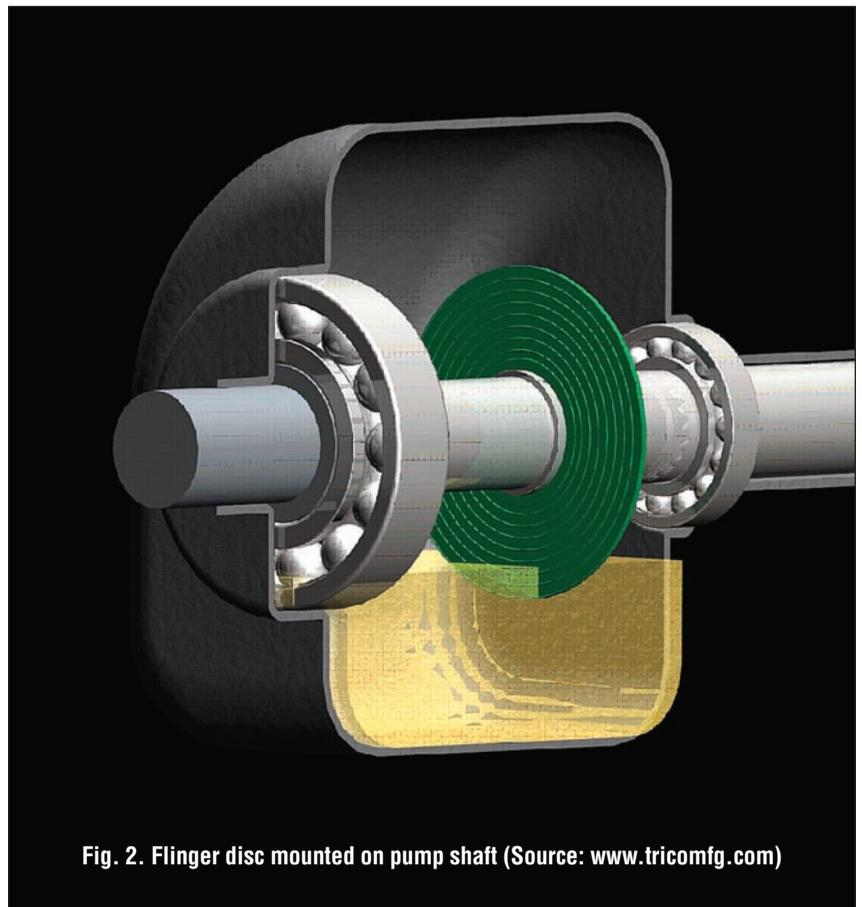
Fig. 2. Flinger disc mounted on pump shaft (Source: [www.tricomfg.com](http://www.tricomfg.com))
