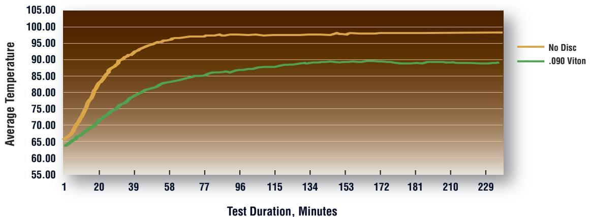
Fig. 4. Flinger disc tests, ISO Grade 32, 3,600 rpm, Average Temp. vs. Time (Source [www.tricomfg.com](http://www.tricomfg.com))
