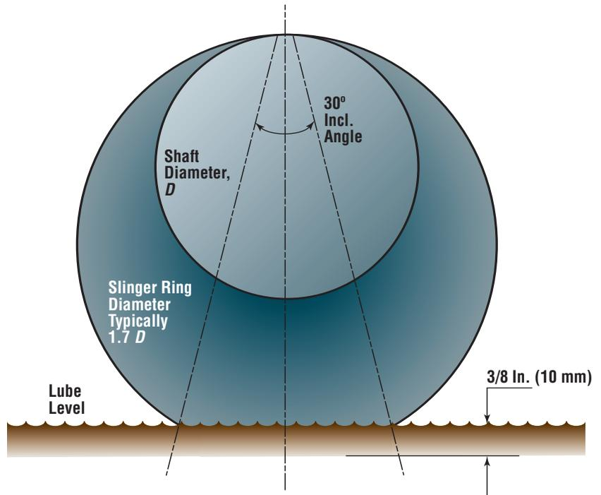
Fig. 1. Oil ring ("slinger ring") and typical dimensions
