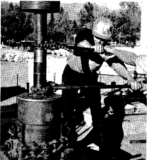
Fig. 7-7. Using Chain Tongs To Make A Tube Joint.
