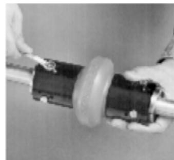
Mount other half of the elastomer element to hubs. Be sure to secure rings to the spacer element if provided. Tighten all cap screws to the recommended cap screw torques in Table 1 and you're done!
