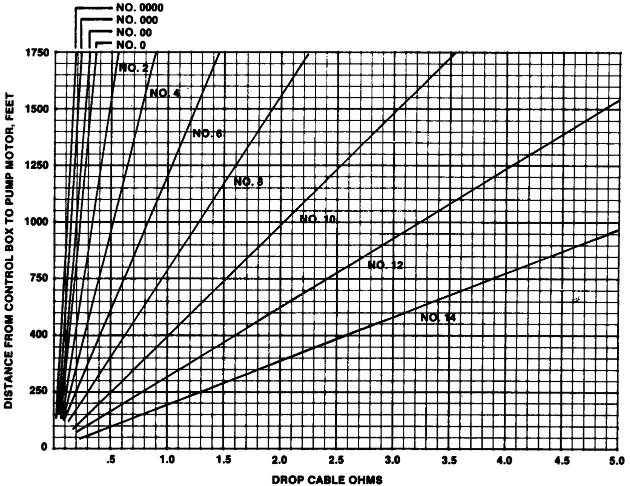
VALUES SHOWN ARE FOR COPPER CONDUCTORS AT 25° C (77° F.)
