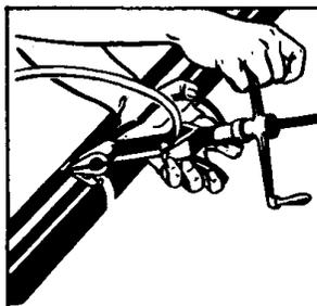
**5** Rotate Tool over Buckle, backing off with Tension Handle throughout entire course of bend. Failure to back off with Tension Handle throughout entire course of bend may result in breaking of Band. There is no loss of tension, as Band released is used up in the bend.
