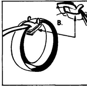
**2** Bring end around object—preferably twice around and through Buckle. Bend end of Band under Buckle (B). For best results, apply Band twice around. Double banding develops at most four times the grip of single banding.
