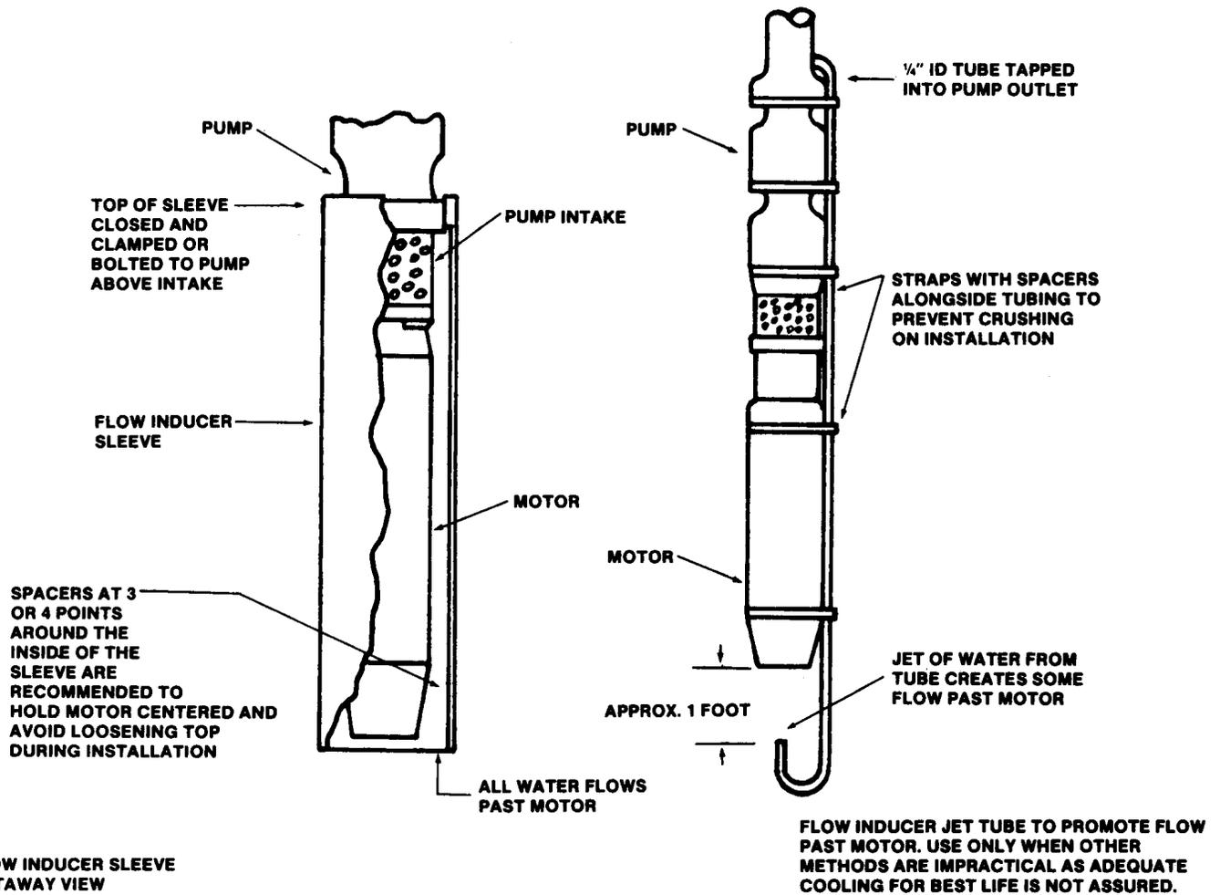
**FIGURE 5. COOLING FLOW INDUCERS**
