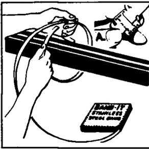
**1** Band may be used from bulk roll as shown, or, for ease of application, cut off about 8' to 10' of Band; hook one end on Buckle (A) then bring the other around object to be banded and through Buckle.
