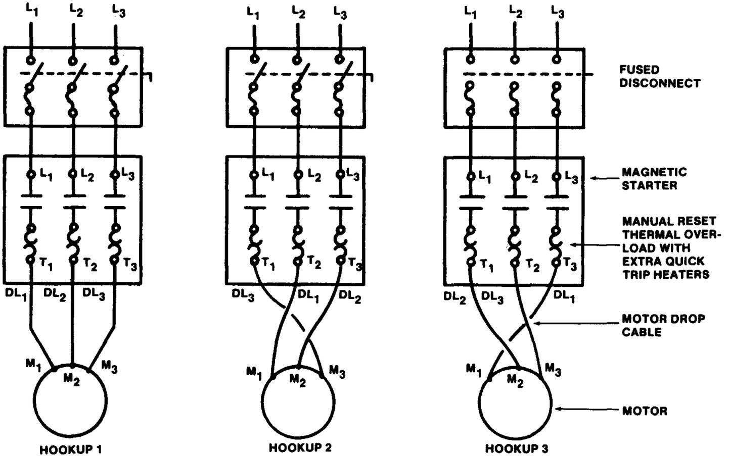
Example: Check for current imbalance for a 230 volt, 3 phase, 60 Hz submersible pump motor, 18.6 full load amps.
