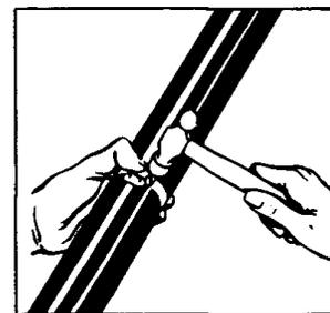
**8** Clinch stub by hammering down Buckle ears, completing BAND-IT CLAMP.
