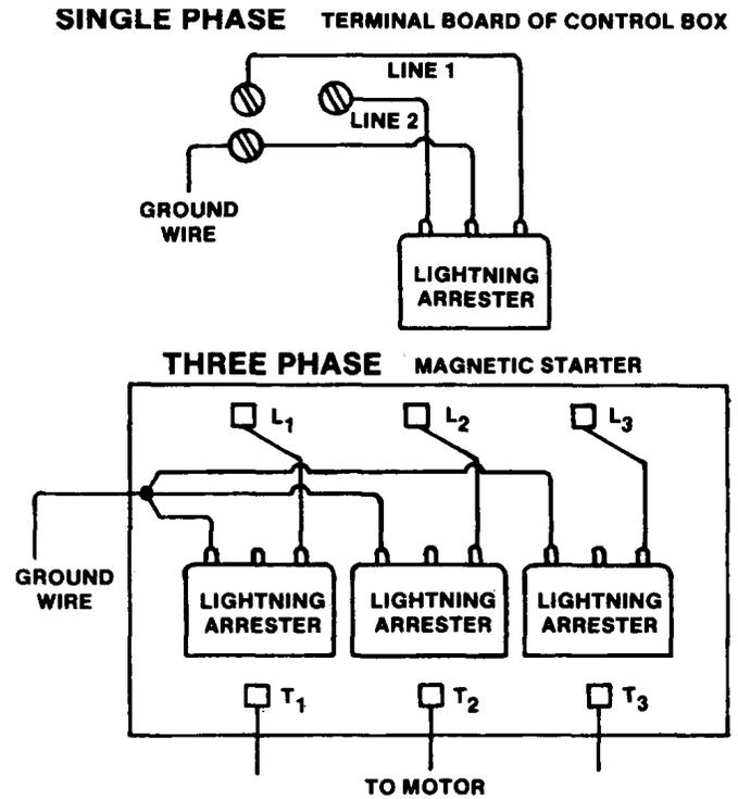
**FIGURE 10. ATTACHMENT OF LIGHTNING ARRESTERS TO SUBMERSIBLE MOTOR POWER LINE.**
