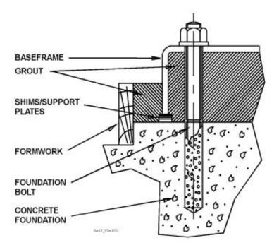
Add or remove shims under the base to level the pump-shaft. The base plate itself does not have to be level.
