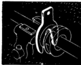
Figure 2 FROG. For locating impeller on shaft.
