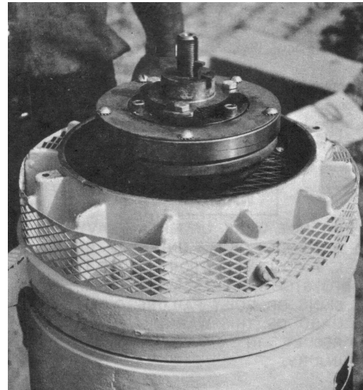
Figure 21. Gib key inserted into top shaft and top drive coupling.
