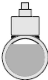
Avoid debris travelling at the bottom of a horizontal pipe.
