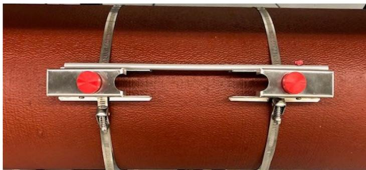
4. Mark the position of the permanent bracket on the pipe. This is the bracket that will not be adjusted and will be used as the reference for the separation distance and alignment. It is your choice which bracket is permanent. With a marker, mark the bracket position by placing the mark directly in front of the stainless side-rail.
