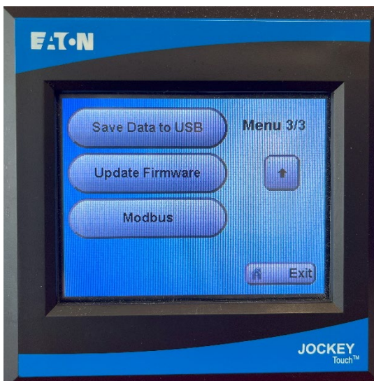
Figure 5 - Eaton Jockey Controller; Main Menu MODBUS Settings
